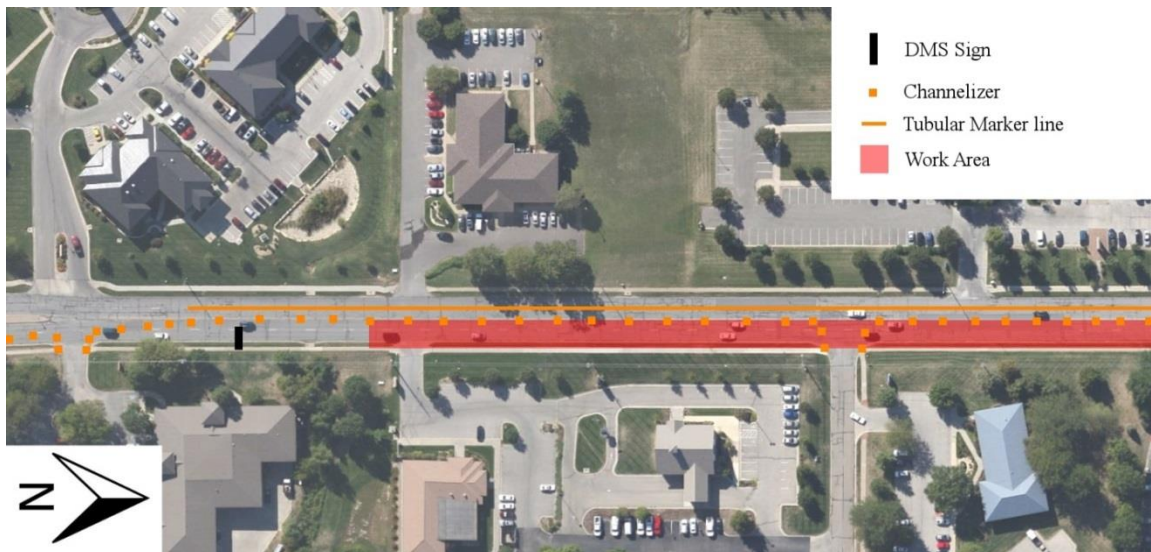
Figure 19. Location 3 Test Area Traffic Control
