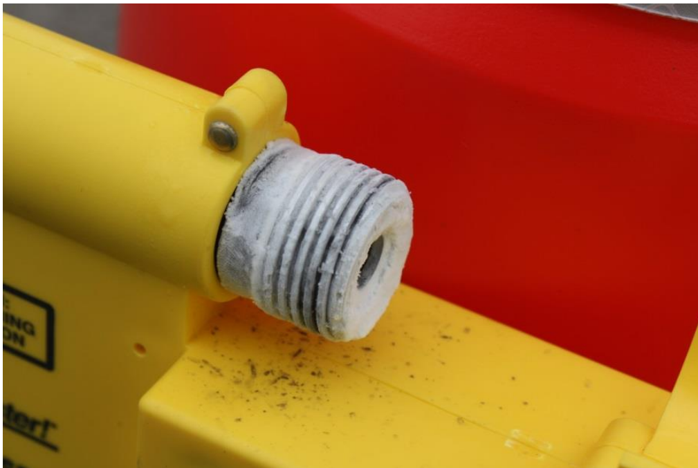
Figure 26. Ice Accumulation on SonoBlaster Nozzle
