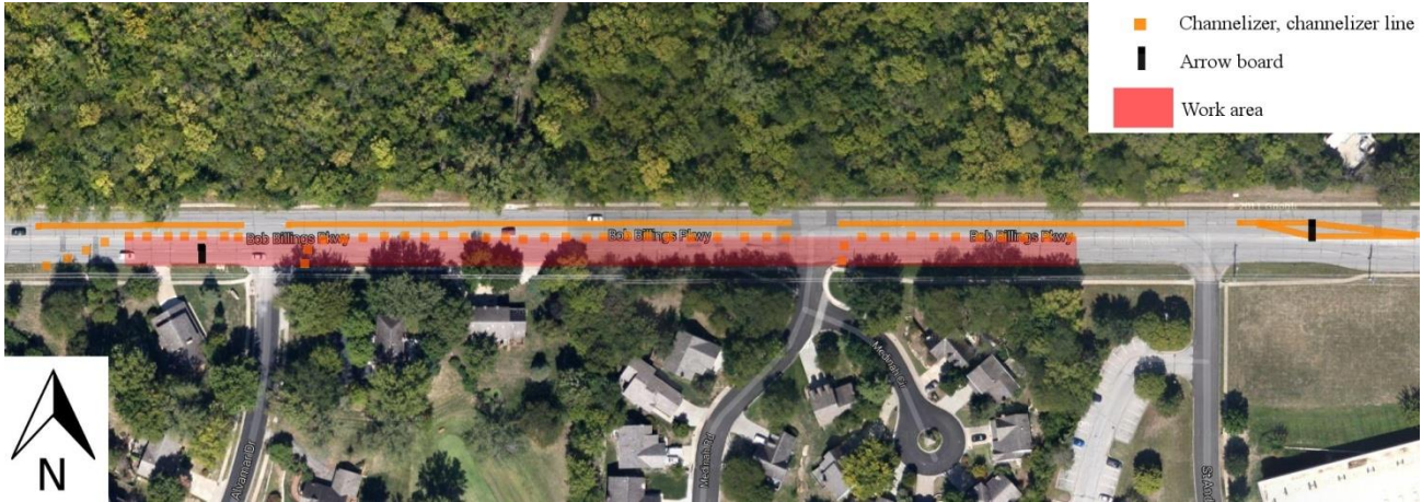
Figure 13. Phase 1 Test Area Traffic Control
